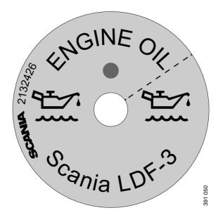
Filling label in the cylinder block.
