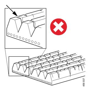
Example of a minor crack in the drive belt. The drive The drive belt has deep cracks and must be renewed. belt can be refitted.
