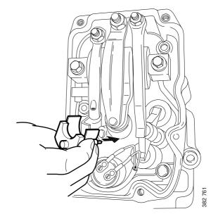
The unit injector is correctly set when the small piston (1) is level with the flat upper surface of the tool. Use a finger to check. You can feel very small differences. See also the illustrations on the next page.
