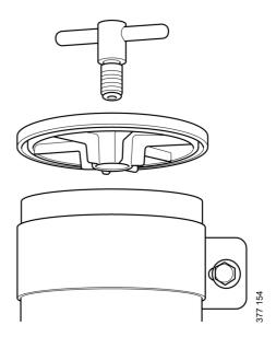
4. Remove the filter and fit the new filter.
