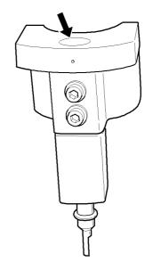
The setting tool piston is above or below the flat upper surface of the tool. Adjust the unit injector.
